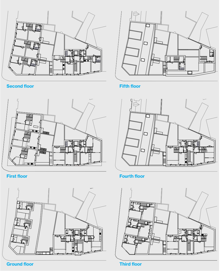
Top, far right Interior and exterior views of Jaccaud-Zein’s Shepherdess Walk (phs: HB, DG). Above, right Shepherdess Walk floor plans, section and axonometric view showing the split-level configuration of living areas that characterises projects by developer Solid Space.
